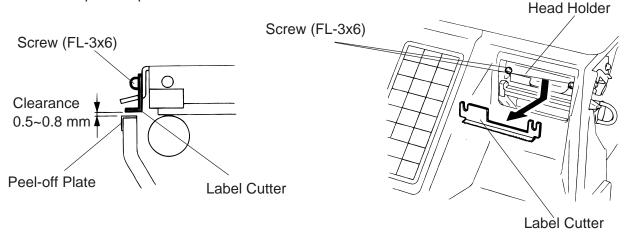
**NOTE:** If the cutter is scratching labels during printing, increase the clearance between the cutter and peel-off plate.
